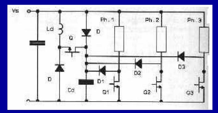
controller for a 4 phase SR motor
