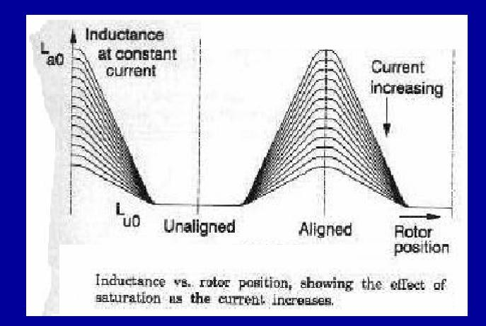
The rotation of the SR motor is achieved by sequentially energizing and de-energizing the phases of the motor
