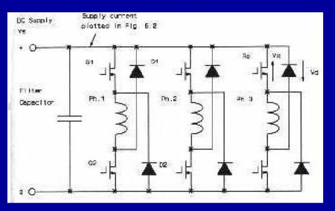
the phases in the SR motor are typically independently controlled
