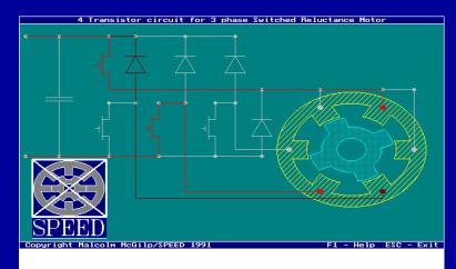
A clockwise sequential excitation of the phases results in a counter clockwise rotation of the SR motor
